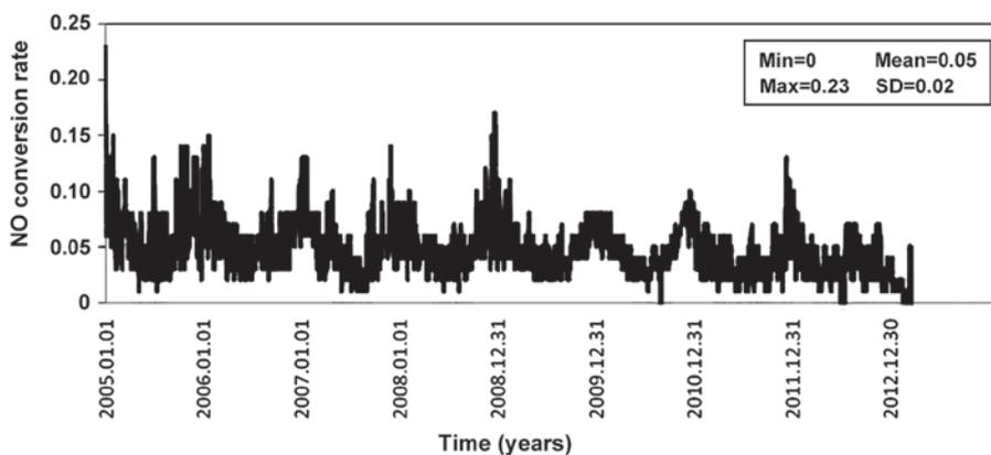
Figure 3. The variation of NO conversion rate during 2004-2012.
