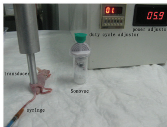
Figure 1. Therapy apparatus for low-frequency US and experimental set-up. US, ultrasound.
