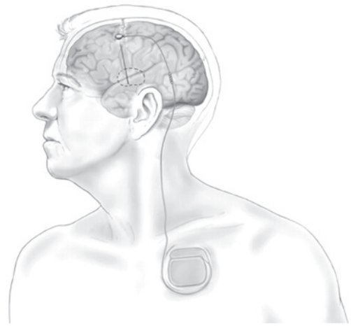
Figure 1. System diagram of deep brain stimulation. The stimulating electrode is implanted by stereotactic neurosurgery and connected to a subcutaneous pulse generator with a wire. This image is provided by David Peace from the Neurosurgery Department, School of Medicine, University of Florida. This image was adapted with permission from Holtzheimer and Mayberg (6).
