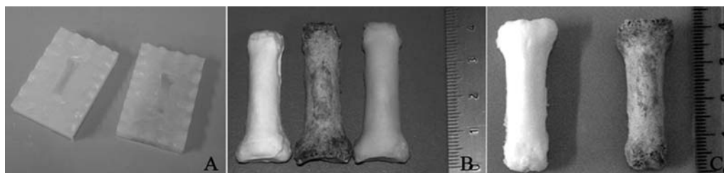
Figure 11. A silicon mould reproducing a human finger phalanx (A) was used to obtain a pre-determined form scaffold. Comparison of human phalanx bone (center) with replicas obtained using PCL (left), or resin (right) (B). Using a mould 8% larger than the original structure, the size of the PCL phalanx was comparable to the one of native bone.
