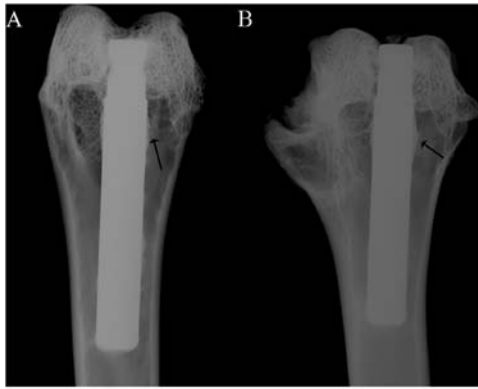
Figure 6. Typical radiographs of Ti6Al4V and Ti35Nb2Ta3Zr alloys at 12 weeks after rod implantation. The new bone formed around the rod is indicated by arrows. (A) Ti6Al4V and (B) Ti35Nb2Ta3Zr.
