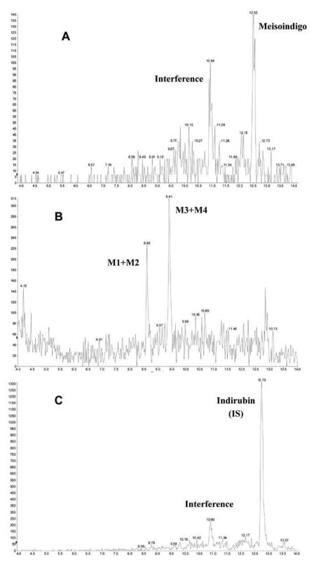
Figure 5. MRM chromatograms for (A) meisoindigo at lower limit of quantitation (1.0 ng/ml), (B) its reductive metabolites at lower limit of quantitation (0.5 ng/ml), and (C) indirubin (internal standard, 100 ng/ml) in rat plasma.
