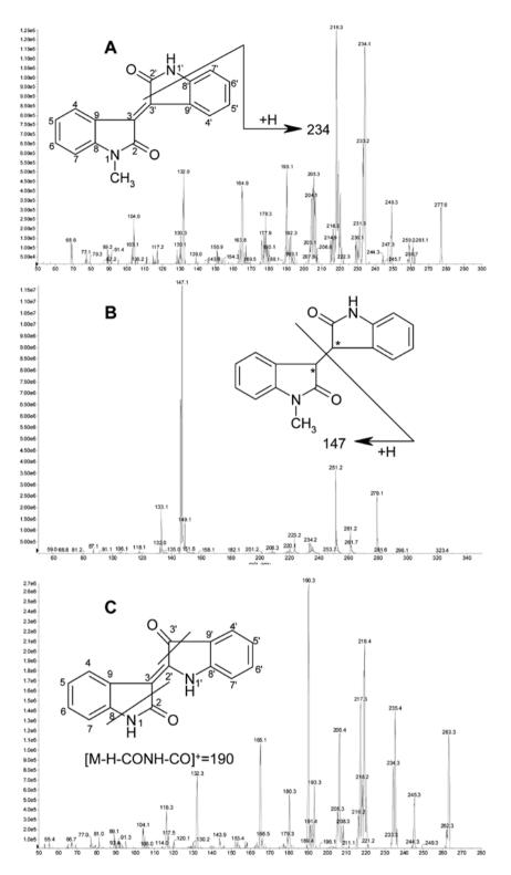
Figure 4. MS/MS spectra of protonated meisoindigo at m/z 277 (A), its reductive metabolites at m/z 279 (B), indirubin (internal standard) at m/z 263 (C), and the proposed origin of key product ions.
