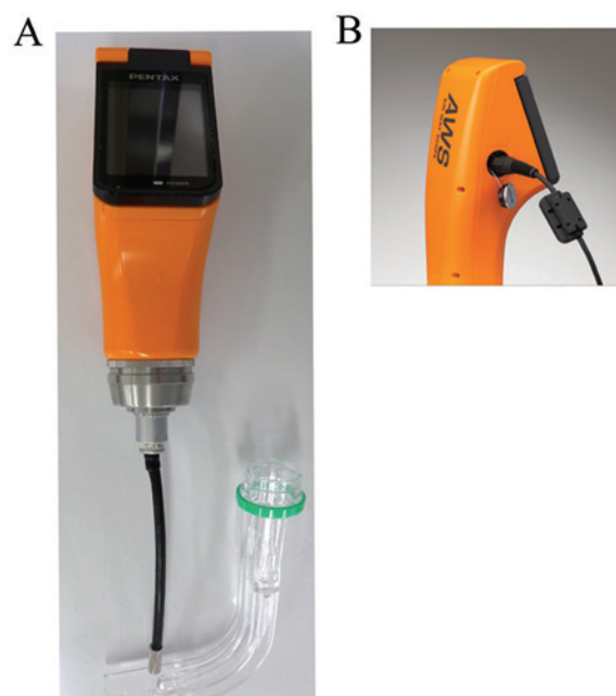
Figure 1. Airwayscope™ (Ricoh, Tokyo, Japan). (A) Frontal and (B) lateral view.
