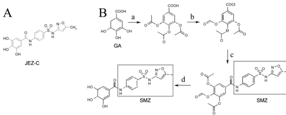
Figure 1. (A) Chemical structure of JEZ-C. (B) JEZ-C synthesis route. Reagents and conditions: (a) Acetyl oxide, oil bath, 120°C; (b) SOCl<sub>2</sub>, oil bath, 80°C; (c) SMZ, THF, Pyridine, ice bath; (d) HCl, THF, 60°C. JEZ-C, 3,4,5-trihydroxy-N-[4-[(5-methylisoxazol-3-yl)sulfamoyl]phenyl]benzamide; SMZ, sulfamethoxazole; THF, tetrahydrofuran.
