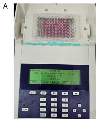
Figure S1. TC-HT treatment utilizing a modified PCR machine and temperature measurements conducted with a thermocouple. (A) Image of the TC-HT controller setup. (B) The thermocouple was inserted into the culture medium and its needle touched the surface where the cells were located to measure the actual temperature experienced by the cells. TC-HT, thermal cycling-hyperthermia.
